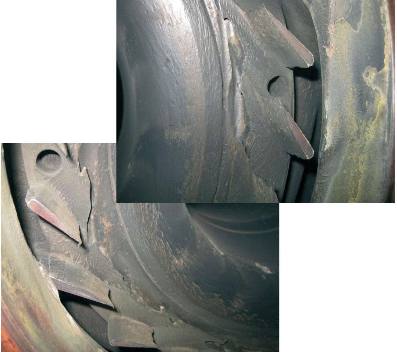
Fig. 6: Worn nozzle ring caused by abrasive particles
