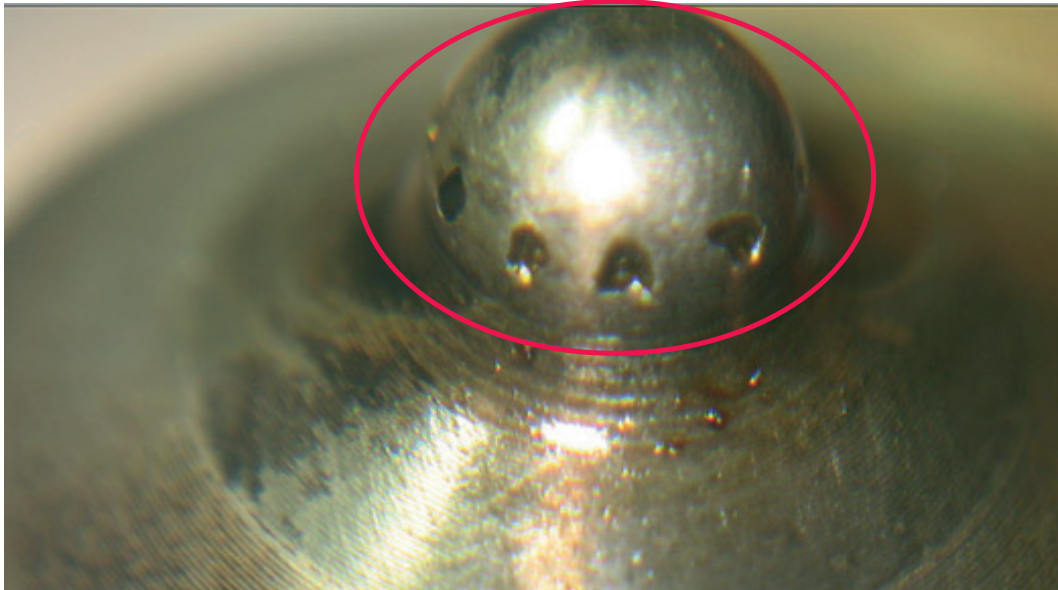
Fig. 4: Abrasive wear has changed the shape and size of the injector holes
